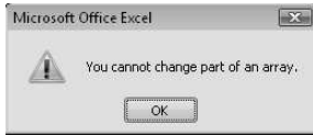
Figure 14-6: Excel's warning message reminds you that you can't edit just one cell of a multicell array formula.
