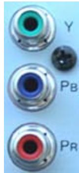
(ခ) component video terminal (Green-Y, Blue-P B , Red-P R color three phono jack)
